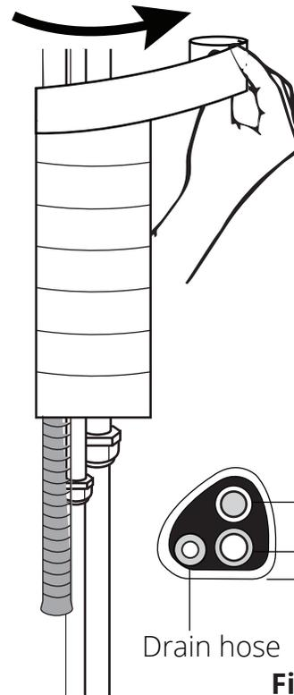
Wrapping the piping upward will prevent rain/moisture from seeping into the overlaps of the tape
