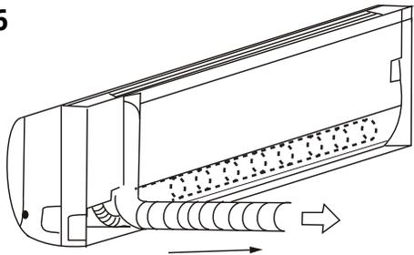
3. Now, you will need to lightly tape the refrigerant piping and drain pipe together in a bundle, using electrical tape, making sure that the drain pipe is at the bottom. **DO NOT** tape the ends of the piping (connectors). Refer to Fig 5.7 and the image below for the correct orientation of the piping when taping.
