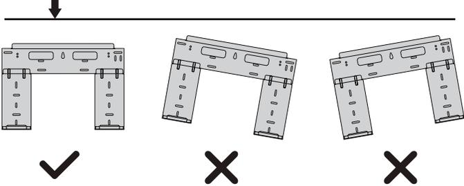
**NOTE:** Use a level in order to ensure your mounting plate is mounted to the wall with the correct orientation shown above.
